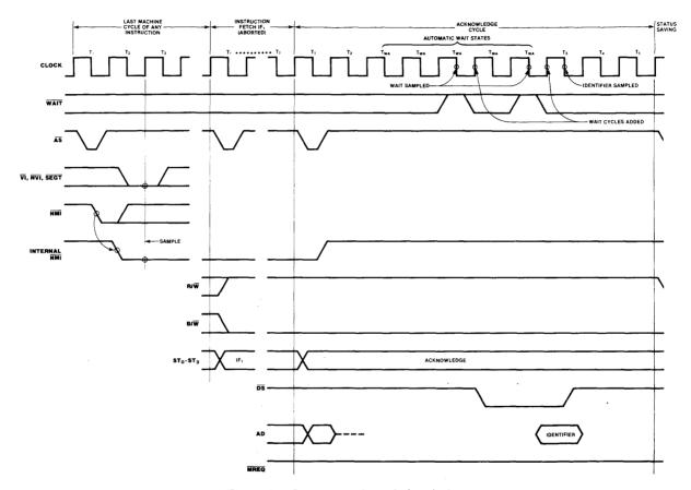
Figure 6.9 Interrupt acknowledge timing.
