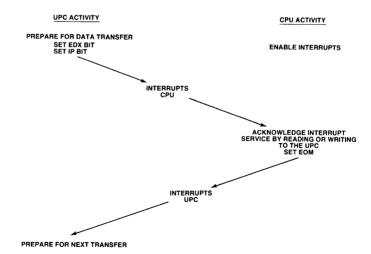
Figure 13.30 Typical master CPU-UPC data transfer protocol.
