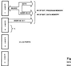
Figure 13.5 Z8 configuration with interface to 4K bytes of external memory.
