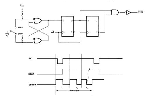
Figure 10.3 Z8000 single-step circuit using the STOP input.
