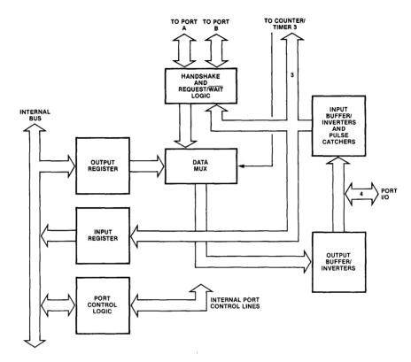
Figure 12.10 CIO port C block diagram.
