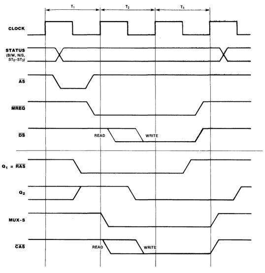
Figure 11.10 Timing of the RAS and CAS signals for dynamic RAM memory accesses.
