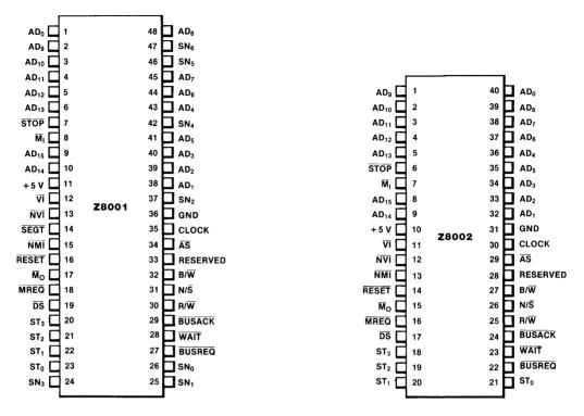
Figure 1.13 Z8000 CPU pin diagrams.
