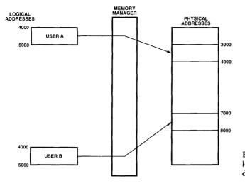
Figure 1.11 Mapping two users' logical addresses into physical addresses.
