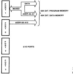
**Figure 13.6** Z8 configuration for memory intensive applications.
