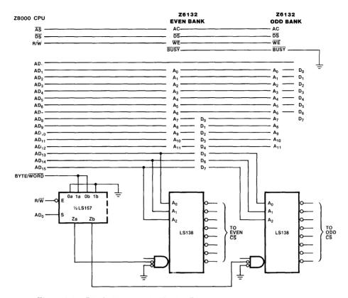
Figure 3.17 Block diagram of a Z8000-Z6132 interface for a 32K word system.
