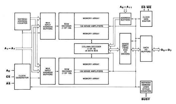
Figure 12.36 Z6132 RAM block diagram.
