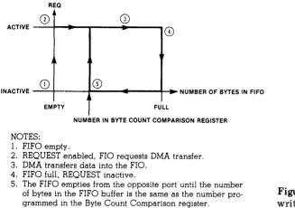
Figure 12.18 DMA-controlled writes to a FIO.
