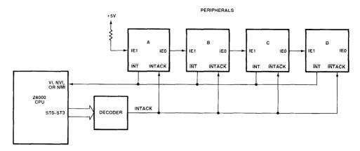
Figure 6.7 Interrupt daisy chain with four devices sharing a common interrupt line.
