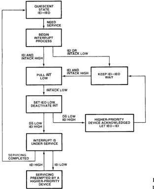
Figure 6.8 Interrupt daisy-chain protocol.
