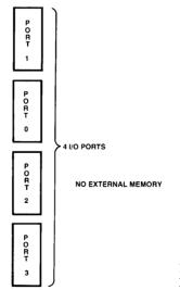
**Figure 13.3 Z**<sup>8</sup> configuration for I/O intensive applications.
