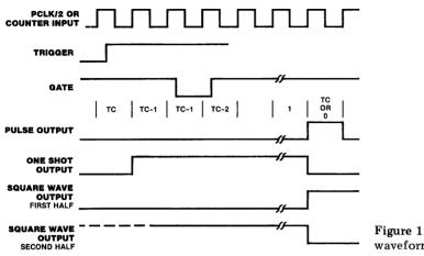
Figure 12.12 Counter/timer output waveforms.
