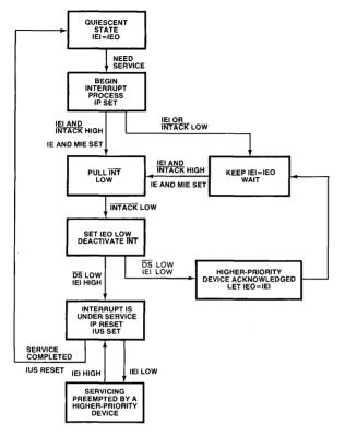
Figure 12.4 Peripheral interrupt protocol.
