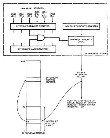
Figure 13.18 Z8 interrupt processing.
