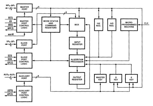
Figure 12.31 Z8068 DCP block diagram.
