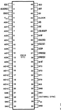
Figure 12.32 Z8016 DTC pin assignments.
