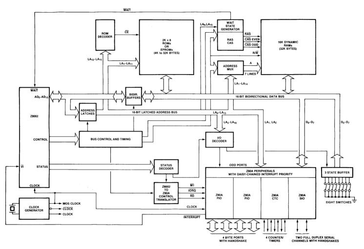
Figure 11.1 Block diagram of a Z8002-based single-board microcomputer.
