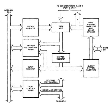
Figure 12.7 CIO ports A and B diagram.
