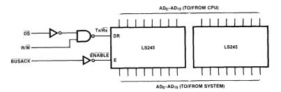
Figure 11.4 Address/data bus buffering using SN74LS245 transceivers.
