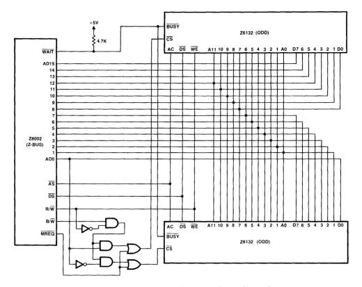
Figure 3.16 Z8002-Z6132 interface logic for a 4K word system.
