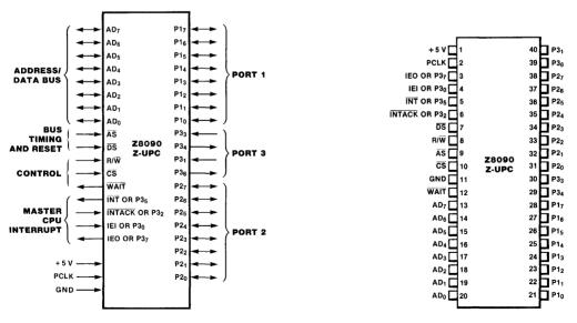
Figure 13.22 Z8090 UPC pin assignments.
