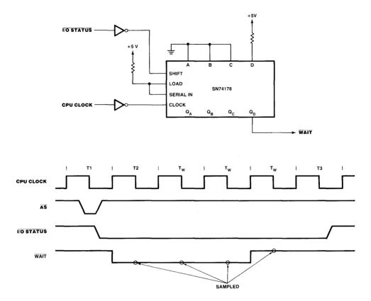
Figure 5.12 Generation of three wait states with a shift register.
