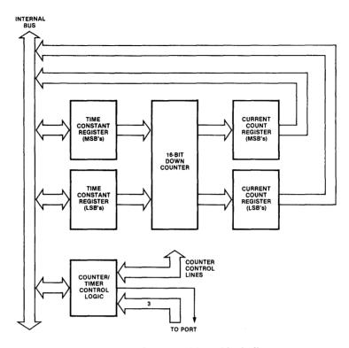
Figure 12.11 CIO counter/timer block diagram.
