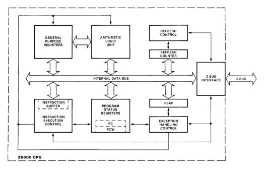
Figure 1.4 Z8000 CPU functional block diagram.
