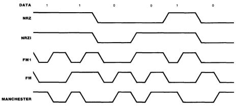
Figure 12.26 Data encoding in the SCC.
