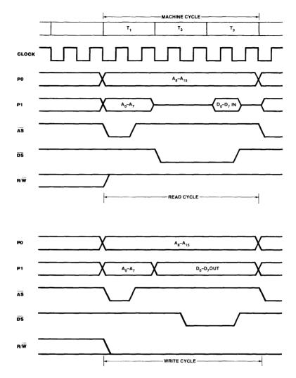
Figure 13.13 Z8 external memory interface timing.
