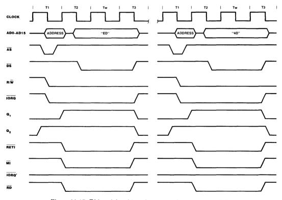
Figure 11.15 Z80 peripheral interface return from interrupt (RETI) timing.
