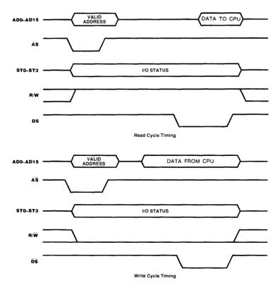
Figure 4.2 CPU-peripheral data transfer timing.
