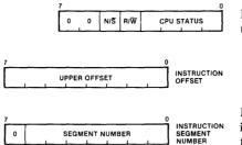
Figure 9.18 Bus cycle status register.
