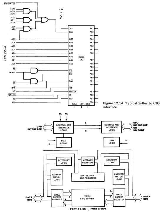
Figure 12.15 Z8038 FIO block diagram.
