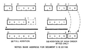
Figure 9.15 Example of address translation process illustrated in two ways.
