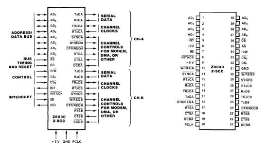
Figure 12.24 Z8030 SCC pin assignments.
