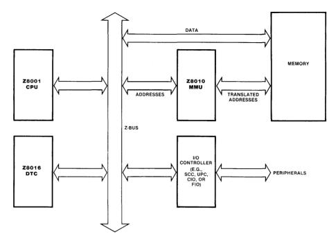
Figure 9.4 Z8010 MMU in a Z8001 system.
