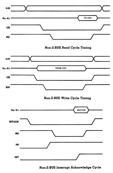
Figure 12.16 Nonmultiplexed bus interface timing.
