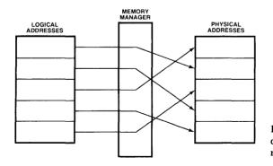
Figure 1.10 Mapping logical addresses to physical addresses using a memory manager.
