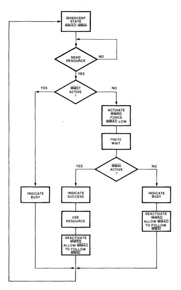
Figure 7.7 Multi-microprocessor resource-sharing protocol.
