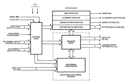
Figure 12.29 Z8065 BEP block diagram.
