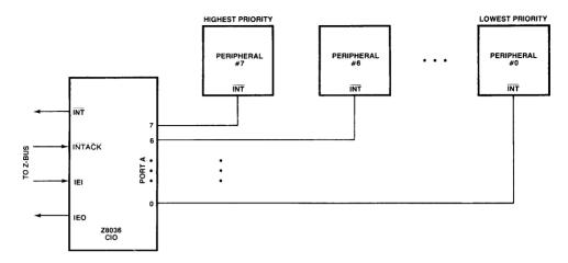
Figure 12.9 CIO as an interrupt controller.
