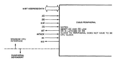
Figure 12.1 Z-Bus peripheral interface signals.
