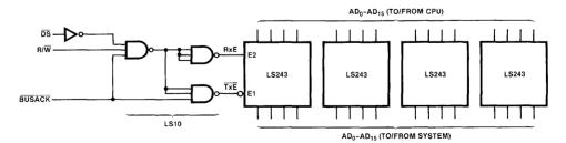
Figure 11.3 Address/data bus buffering using SN74LS243 transceivers.
