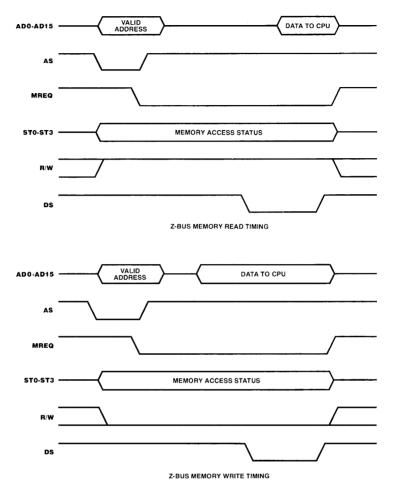
Figure 3.9 Z-Bus memory transaction timing.
