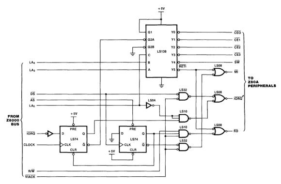
Figure 11.12 Interfacing Z80 peripherals to the Z-Bus.
