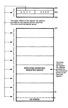
Figure 13.11 Z8 register pointer.
