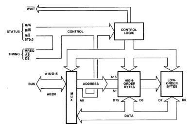
Figure 3.7 Typical Z8000 memory interface block diagram.
