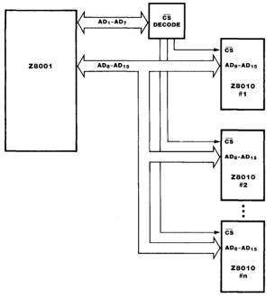
Figure 9.21 Decoding address lines to generate chip selects for MMUs.
