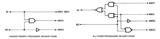
Figure 7.8 Logic for mapping the Z-Bus resource-sharing signals to the Z8000 CPU MO and MI pins.
