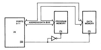
Figure 13.9 Using the  $\overline{DM}$  signal to segregate external program and data memory.
