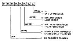
Figure 13.28 Data Transfer Control register.
