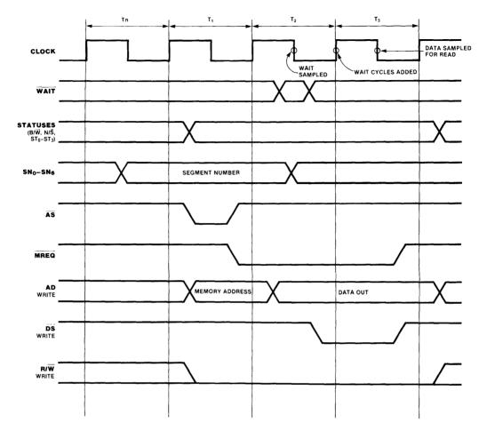
Figure 5.5 Memory write bus transaction timing.
