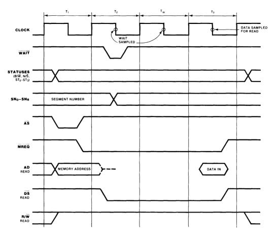
Figure 5.4 Memory read bus transaction timing with one wait state.
