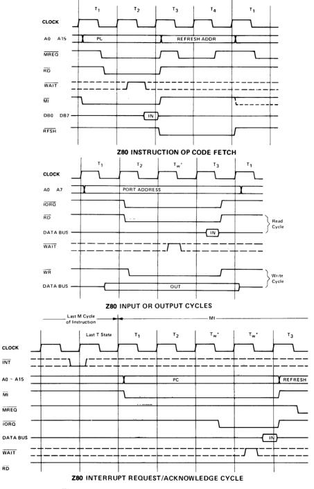
Figure 11.11 Timing of Z80 CPU machine cycles.
