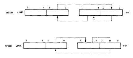
Figure 8.12 Rotate Left Digit and Rotate Right Digit instructions.
