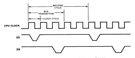
Figure 5.2 Basic timing periods for the Z8000.
