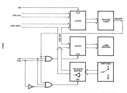
Figure 4.4 Z-Bus interface to a byte peripheral consisting of switches and lamps.
