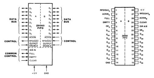
Figure 12.21 Z8060 FIFO pin assignments.
