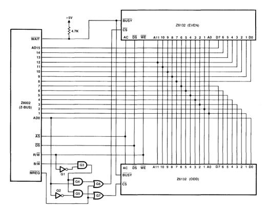
Figure 5.10 Z8002-Z6132 interface logic for a 4K word system.
