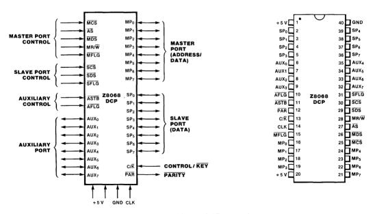
Figure 12.30 Z8068 DCP pin assignments.
