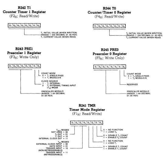
Figure 13.16 Counter/timer control and status registers.
