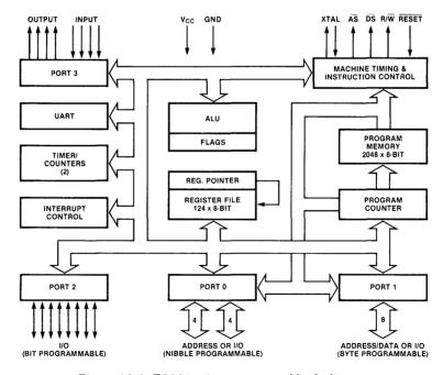
Figure 13.2 Z8601 microcomputer block diagram.
