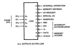
**Figure 11.6** Status decoding with an SN74LS42 decoder.
