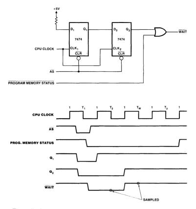
Figure 5.11 Generation of a single wait state with D-type flip-flops.
