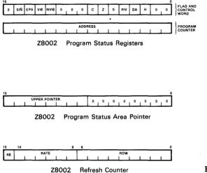
Figure 2.3 Z8002 control registers.
