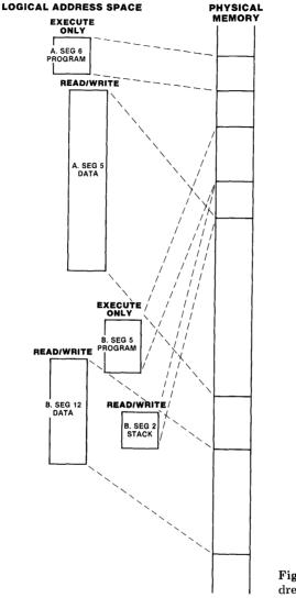
Figure 9.2 Mapping logical addresses to physical addresses.
