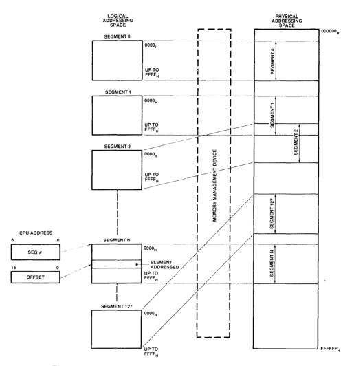
Figure 9.3 Memory mapping of segments with a memory manager.
