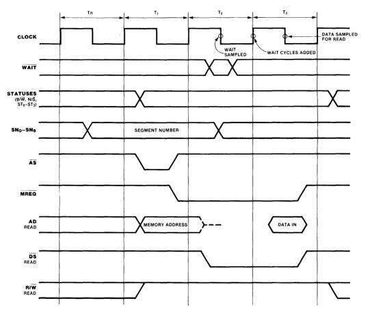
Figure 5.3 Memory read bus transaction timing.
