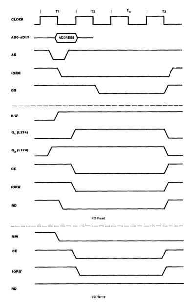
Figure 11.13 Z80 peripheral interfacing read and write timing.
