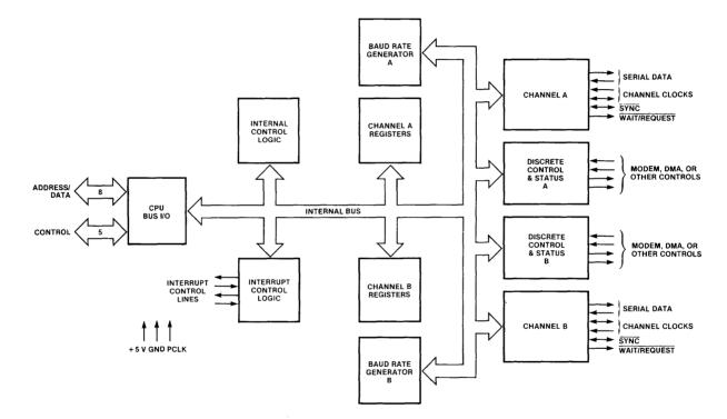
Figure 12.25 Z8030 SCC block diagram.
