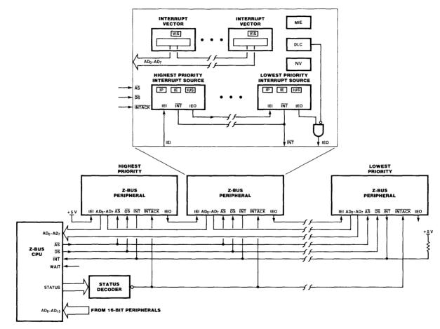
Figure 12.3 Z-Bus peripheral interrupt structure.
