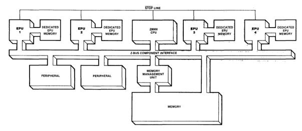
Figure 10.1 Typical Z8000 configuration with 10 EPUs.
