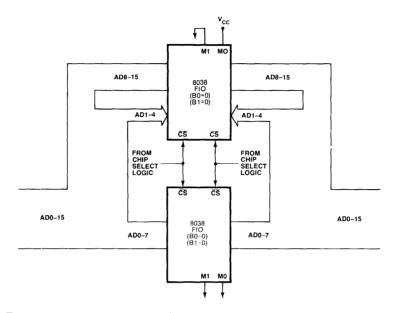
Figure 12.23 16-bit-wide buffer between two Z-Bus processors using Z8038's.
