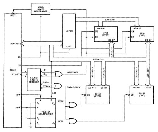
Figure 3.18 Z8002 interface to 2716's and Z6132's.
