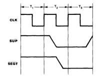
Figure 9.20 Timing of SUP and SEGT signals.
