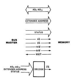
Figure 3.8 Z-Bus signals for CPUmemory transactions.
