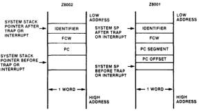
Figure 6.2 Saved program status on the system stack.
