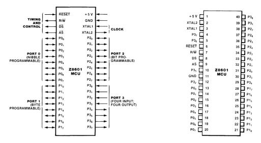
Figure 13.1 Z8601 microcomputer pin assignments.
