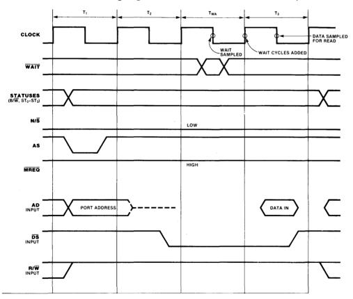
Figure 5.6 I/O read bus transaction timing.
