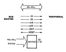
Figure 4.1 Z-Bus signals for CPUperipheral data transfers.
