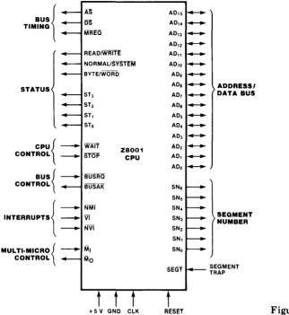
Figure 1.8 Z8001 pin functions.
