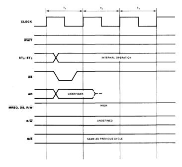
Figure 5.8 Internal operation bus transaction timing.
