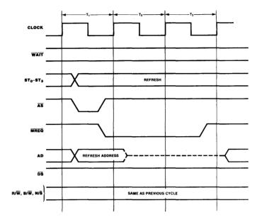
Figure 5.9 Memory refresh bus transaction timing.
