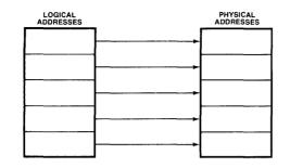
Figure 1.9 Example of identical logical and physical memory addresses.
