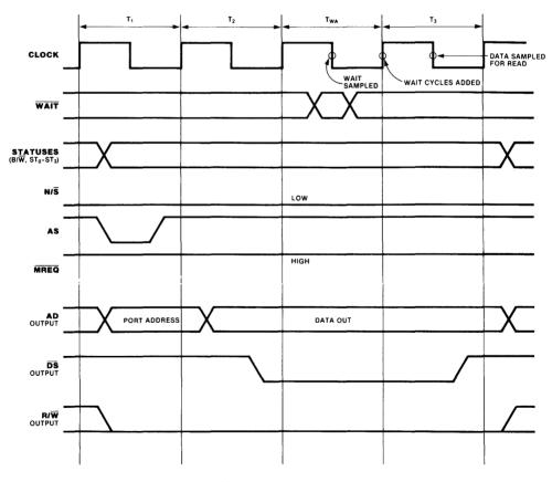
Figure 5.7 I/O write bus transaction timing.
