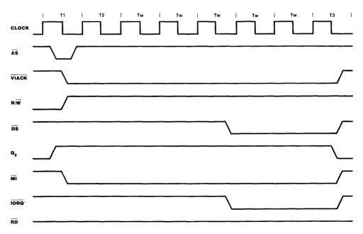
Figure 11.14 Z-80 peripheral interface interrupt acknowledge timing.
