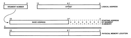
Figure 9.7 Generation of a physical address from a logical address.
