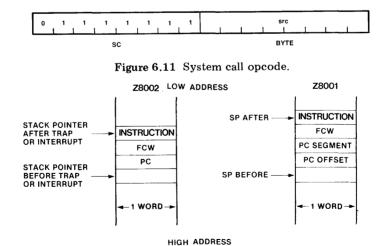
Figure 6.12 Saved program status for a system call trap.
