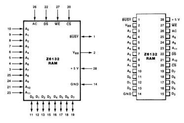
Figure 12.35 Z6132 Quasi-Static RAM pin assignments.
