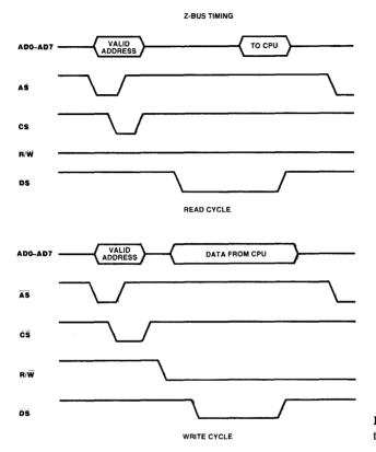
Figure 12.2 Z-Bus to peripheral interface timing.
