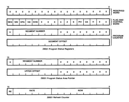
Figure 2.6 Z8001 control registers.
