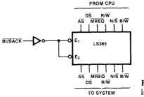
Figure 11.5 Control signal buffering using an SN74LS365 buffer.
