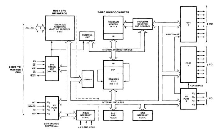
Figure 13.23 Z8090 UPC block diagram.
