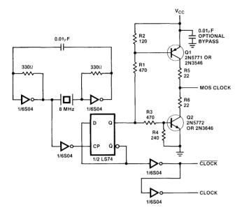
Figure 1.14 Z8000 CPU clock driver circuitry.
