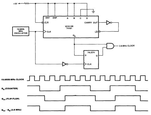
Figure 11.2 Generation of a 3.9-MHz clock from a 19.6608-MHz oscillator.
