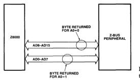
Figure 4.3 CPU-peripheral byte data transfers.
