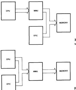
Figure 12.33 System with the DTC using physical memory addresses.
