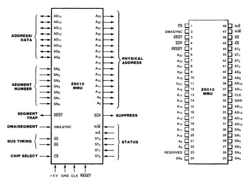
Figure 9.5 Z8010 MMU pinout.
