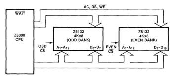
Figure 3.15 Block diagram of a Z8000-Z6132 interface for a 4K word system.
