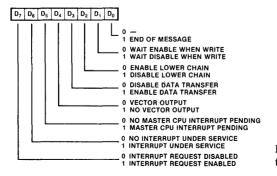
Figure 13.27 Master Interrupt Control register. **R0 DTC Data Transfer Control Register** Z-UPC register address (Hex): 00
