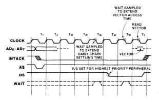
Figure 6.10 Wait states in the interrupt acknowledge cycle.
