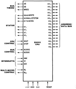
Figure 1.5 Z8002 pin functions.
