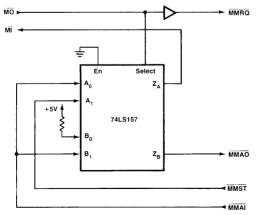
Figure 7.9 Mapping Z-Bus resourcerequest signals to a Z8000 CPU using a 2-to-1 multiplexer.
