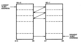
Figure 3.4 Sequencing of bytes in memory.
