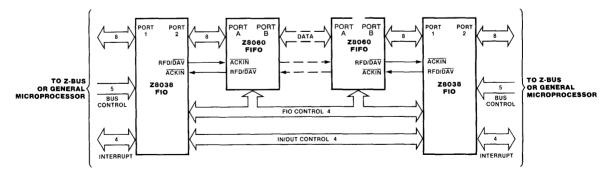
Figure 12.22 512-byte buffer using Z8038's and Z8060's.
