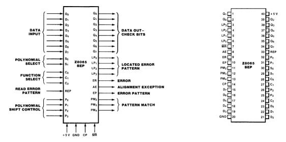
Figure 12.28 Z8065 BEP pin assignments.
